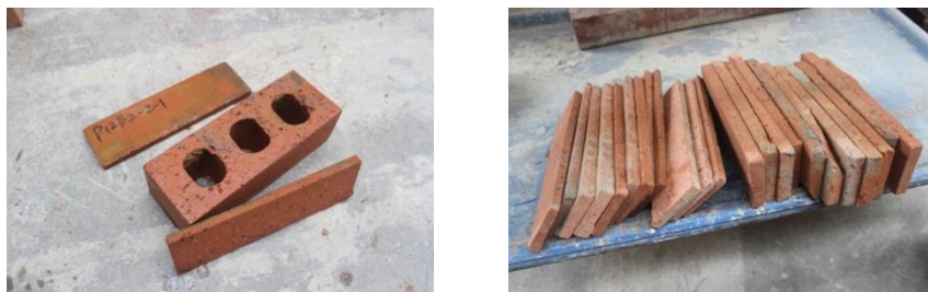
Figure 6. Brick slips obtained by saw-cutting.
