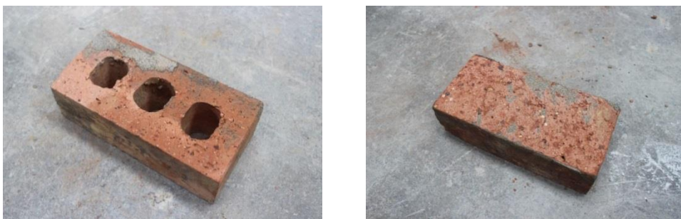
Figure 4 (a). Reclaimed bricks by saw-cutting method.
