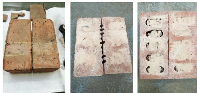
Figure 4 (b). Reclaimed bricks by punching method.
