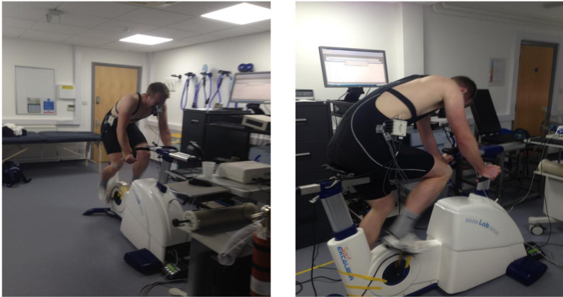
Figure 3.1. Participant performing a 3-min all-out cycling test on an electronically braked cycle ergometer. Note neuromuscular function is also being assessed via peripheral nerve stimulation and electromyography of the quadriceps.
