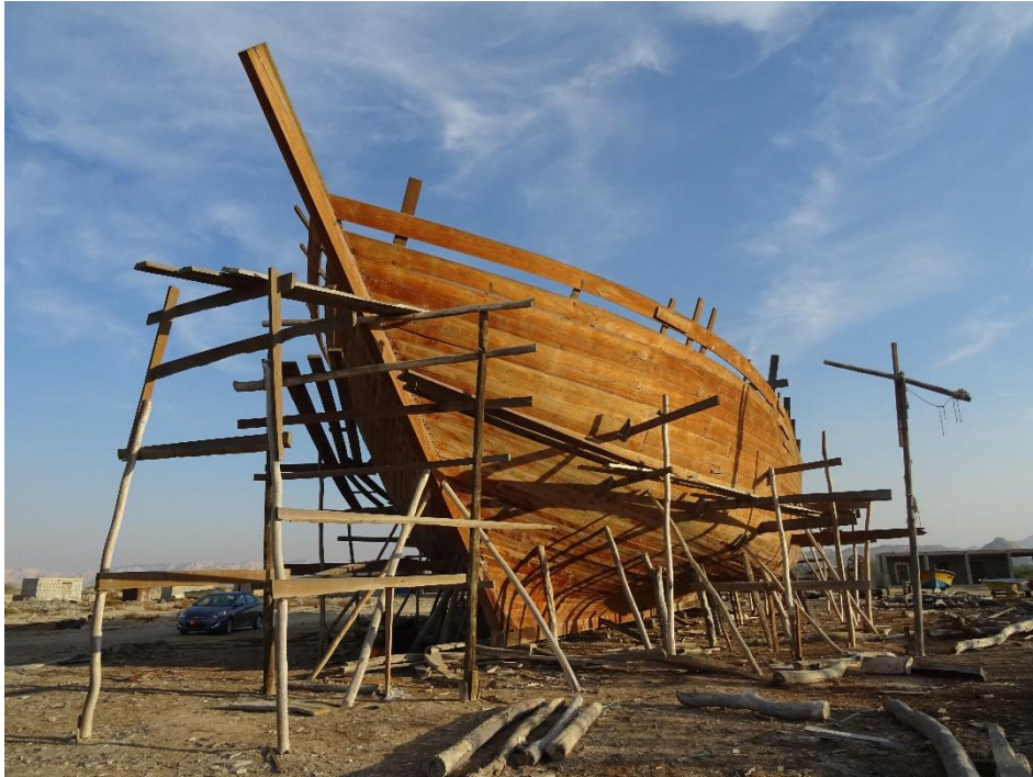
(Fig. 3.4) Building a traditional wooden ship ( Lenj ) near Laft village. Photo taken in November 2016. (Image: Manami Goto)
