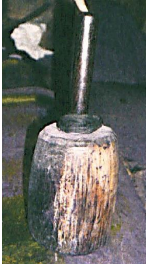
(Fig. 5.2) A wooden hammer used to hit a fabric to make its surface shiny (Al Shomely 2016, 63). Photo reproduced from Al Shomely (ibid.).
