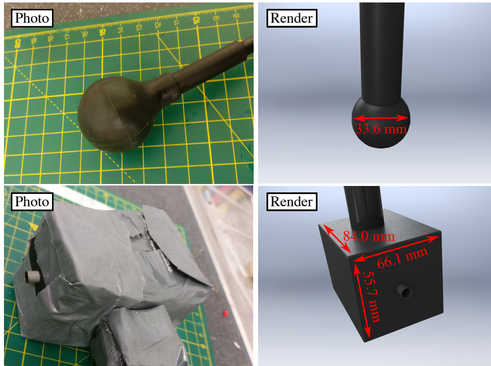
Figure 3.3: Photos and renders of the two sources. Top is the normal Neptune Sonar D70 transducer and bottom is the EVA foam wrapped D70 transducer. Left are photos of the devices on a 1 by 1 cm grid and right is the graphical representations of these devices with the dimensions given. Measurements of the diameter of the ball D70 has \pm 0.1 mm error and the dimensions of the wrapped D70 has \pm 0.5 mm error.
