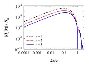
Fig. 3 Spectrum of two-dimensional leakage field determined using (7) for d = 2a,  $\mu_r >> n$  and constant defect width for different defect depths.
