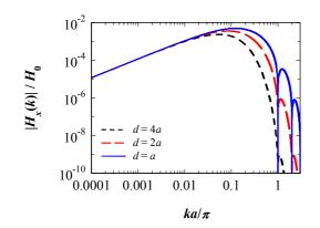
Fig. 4 Two-dimensional spectrum of leakage field determined using (7) for *b* = 4*a* and  $\mu_r >> n$  for different surface separations *d*.
