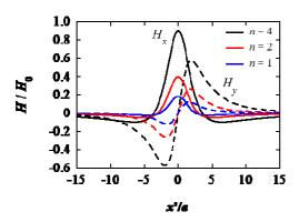
Fig. 2 Longitudinal (solid lines) and vertical (dashed lines) leakage field components for d = 2a and  $\mu_r >> n$ .
