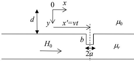
Fig. 1 Two-dimensional geometry used in the theory with a defect moving at velocity  $v$  with respect to the reference coordinate system corresponding to the fixed position of the flux-sensitive sensing element.
