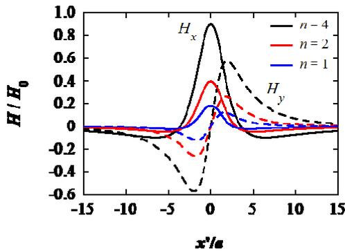
Fig. 2 Longitudinal (solid lines) and vertical (dashed lines) leakage field components for  $d = 2a$  and  $\mu_r \gg n$ .
