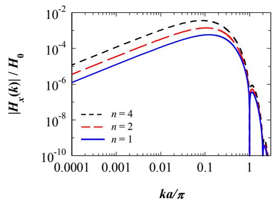
Fig. 3 Spectrum of two-dimensional leakage field determined using (7) for  $d = 2a$ ,  $\mu_r \gg n$  and constant defect width for different defect depths.
