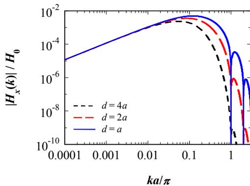
Fig. 4 Two-dimensional spectrum of leakage field determined using (7) for  $b = 4a$  and  $\mu_r \gg n$  for different surface separations  $d$ .
