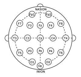
Figure 1. International 10-20 EEG electrode placement system
