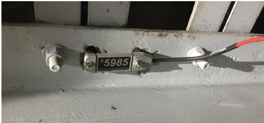
Figure 4.20 Picture for BDI transducers in use on top of a cross beam.
