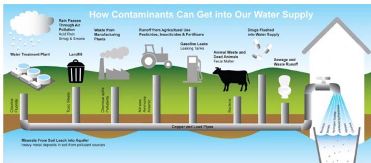
Fig. 1. Schematic diagram of the range of sources of chemical contaminants into the aquatic environment (Source: United Nations World Water Development Report 3: Water in a Changing World).
