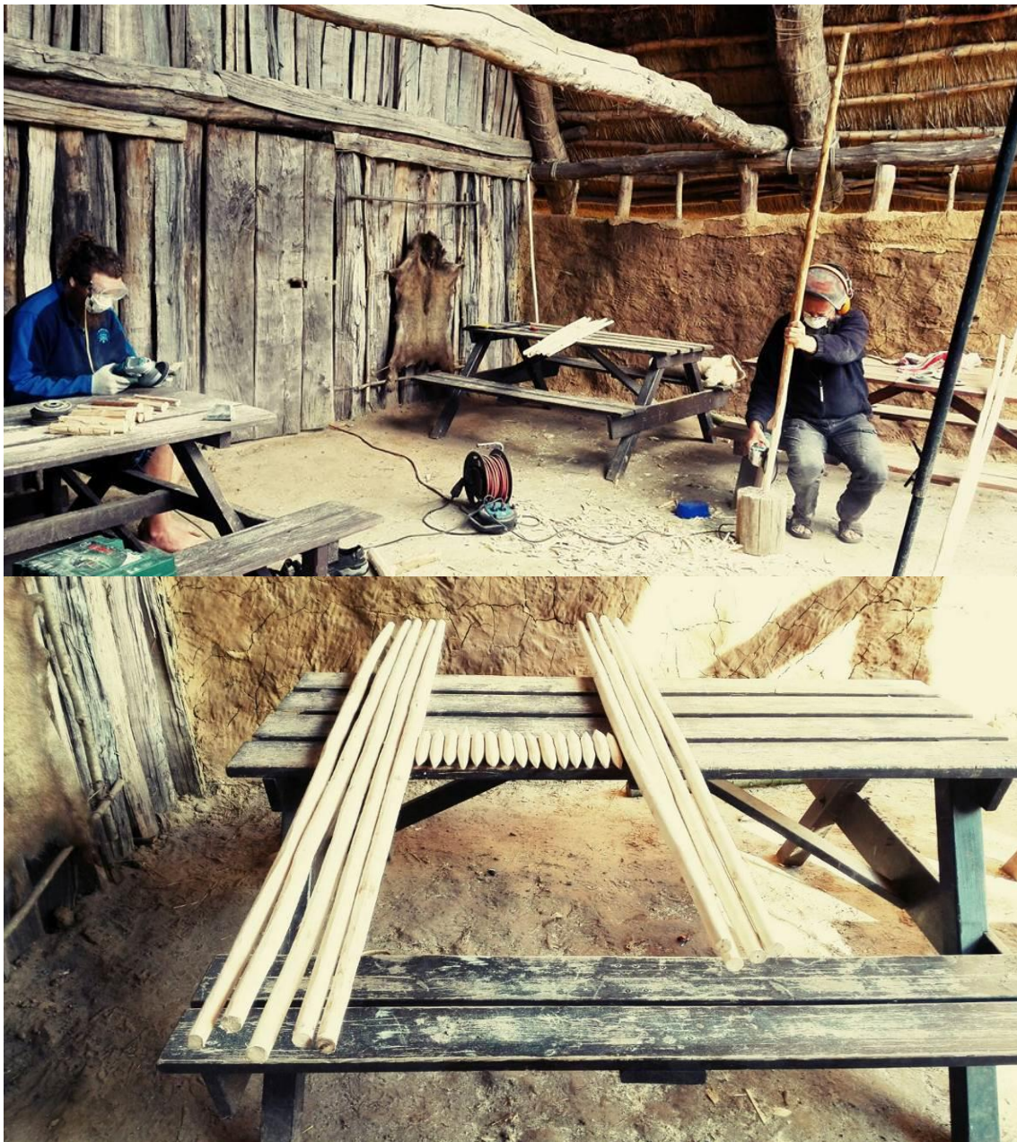
Figure 4.31. Shaft manufacturing process (de-barking and first planning), second set of experiments.
