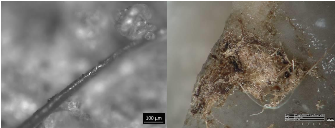
Figure 2.6. Left: animal hair residue. Picture was taken with the OLMil (Olympus BX60) image with manual focus (Z-stack) based on 12 pictures at 100x (2 minutes realisation time). Right: animal flesh residue. Picture was taken with an Hirox- 8700 DM image with an automatically extended focus (Z-stack) based on 27 pictures, at 100x (Low-range objective lens, 20 seconds realisation time). (Image La Porta).
