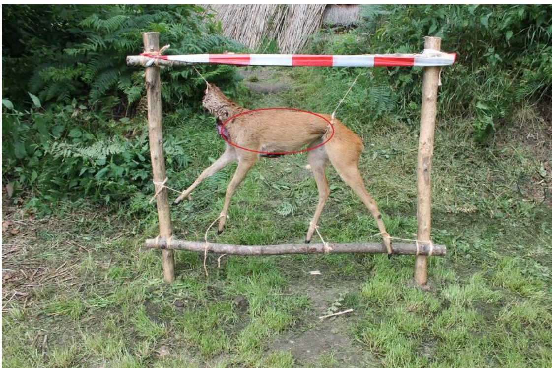
Figure 4.23. Animal target positioned into the frame in a “running position”. The red circle indicates the aiming area.
