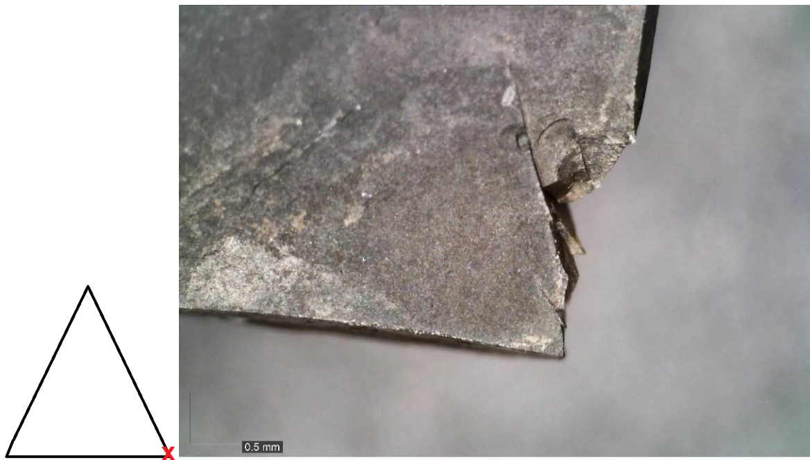
Figure 7.10. Edge-damage (i.e. edge-crushing) due to the presence of a hafting system. DM OM 60x (experiment code: TH-23).
