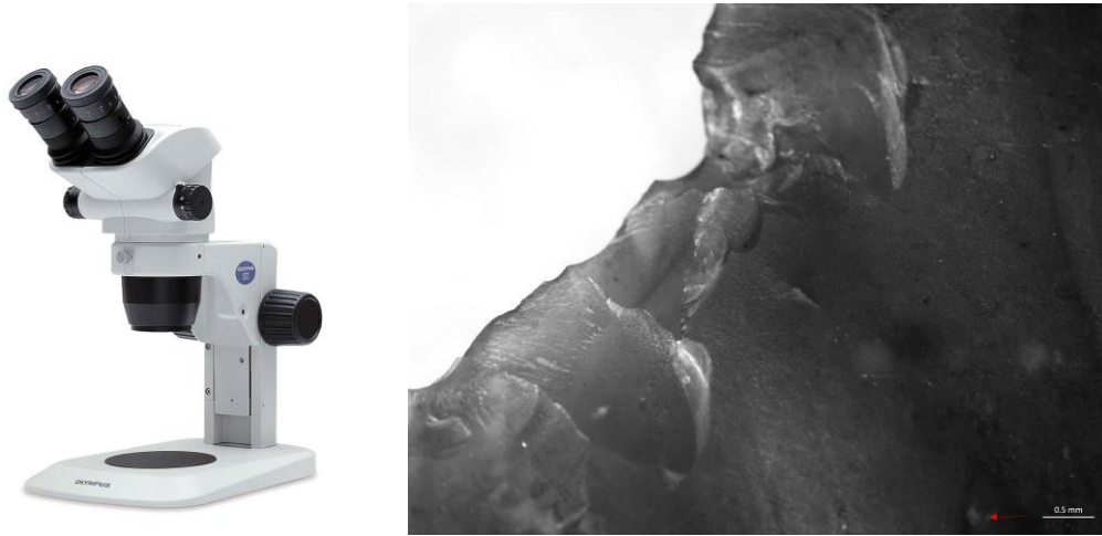
Figure 2.1. Left: The stereomicroscope Olympus SZ61 (located at the Department of Archaeology, University of Exeter). Right: Multiple-fractures observed with the stereomicroscope (OM 25x).
