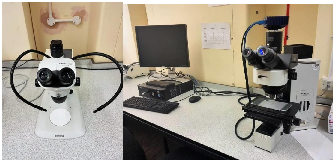
Figure 2.3. The stereomicroscope and the OLMil microscopes located at the Department of Archaeology, University of Exeter. (Image La Porta).
