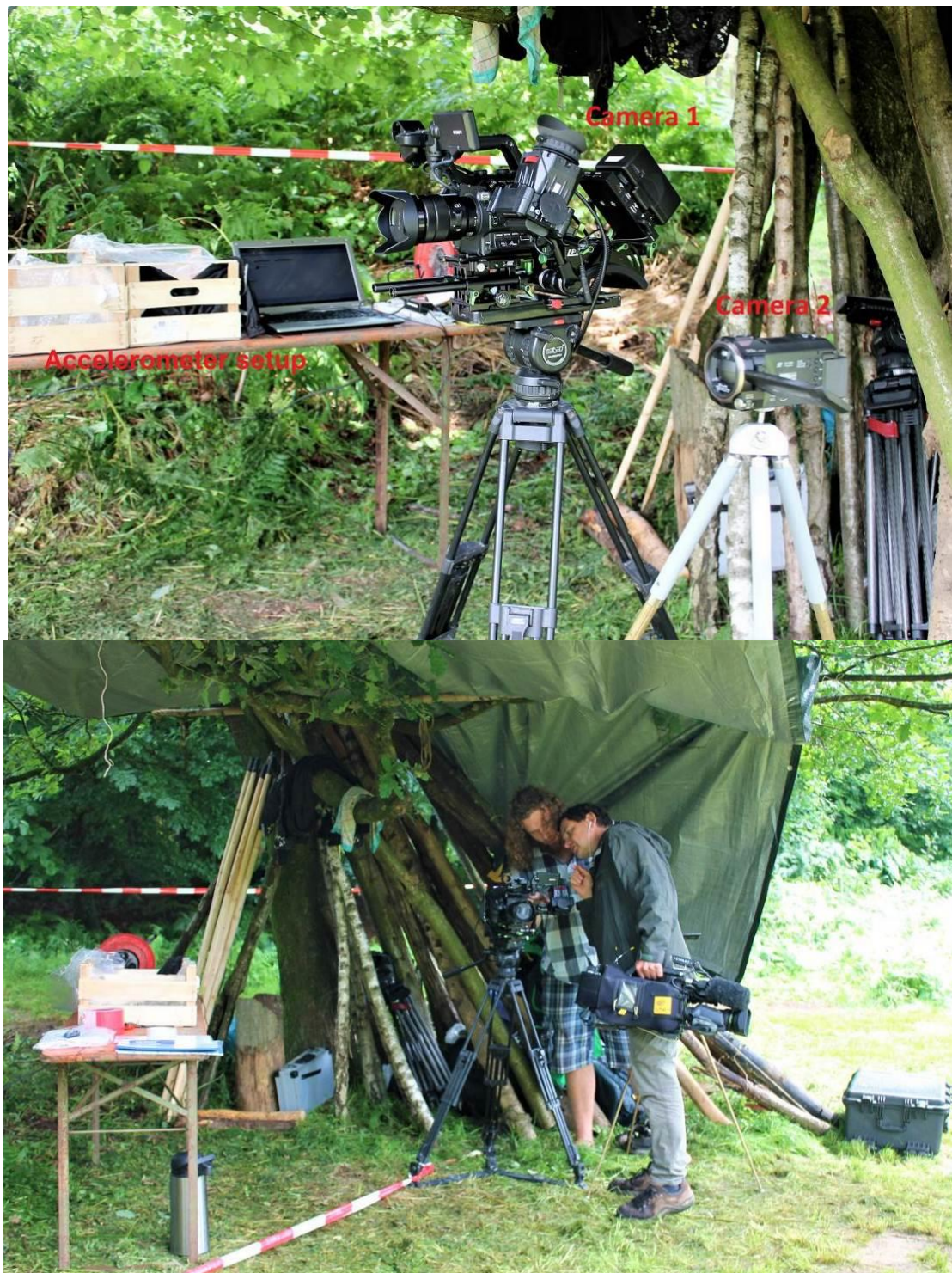
Figure 4.24. Above: Camera setup. Cam1: Sony FS5 XDCAM High-speed Camera; Cam2: Canon Shot SX270 HS; Accelerometer setup. Below: IP and TB mounting the equipment and setting the cameras.
