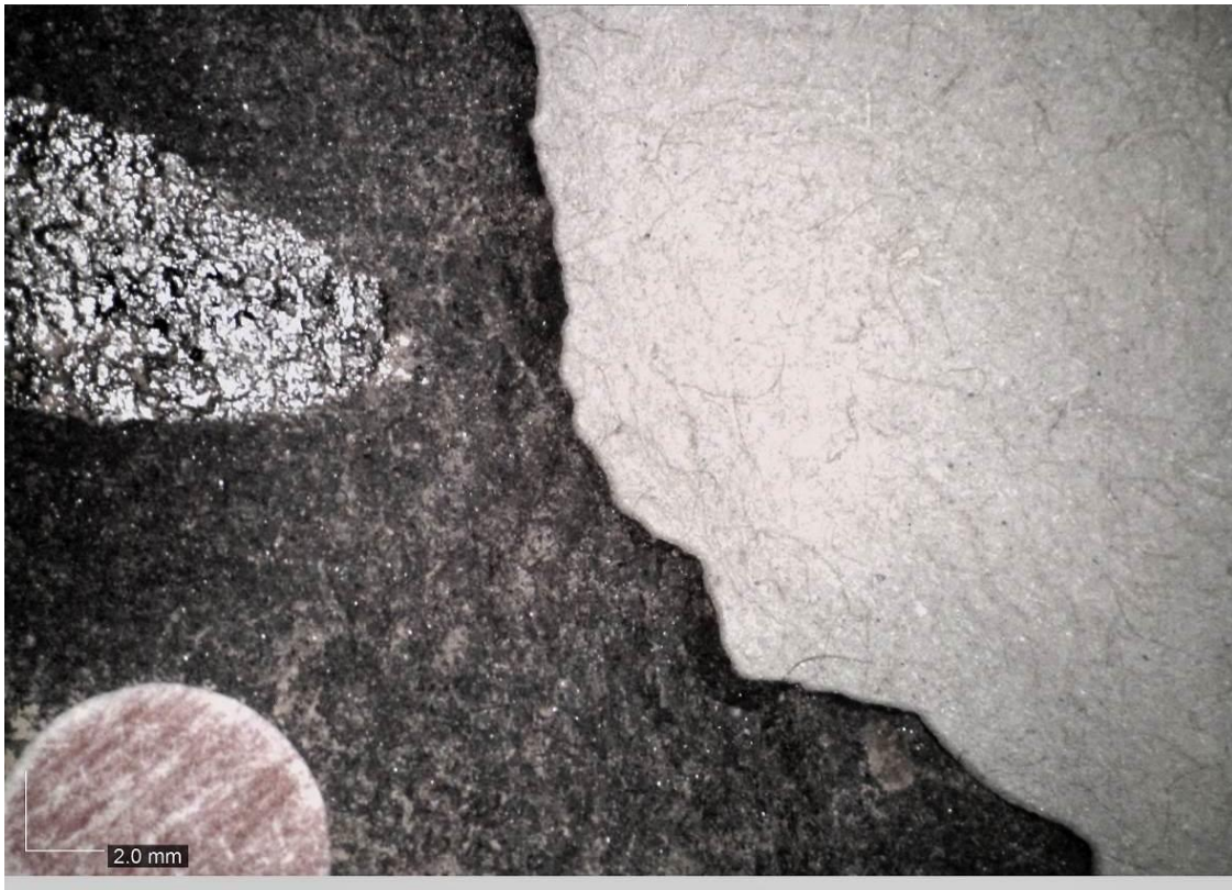
Figure 9.7. Traces of lacquer and sticker, DM OM 13x (Tool ID #rem C 51-70).
