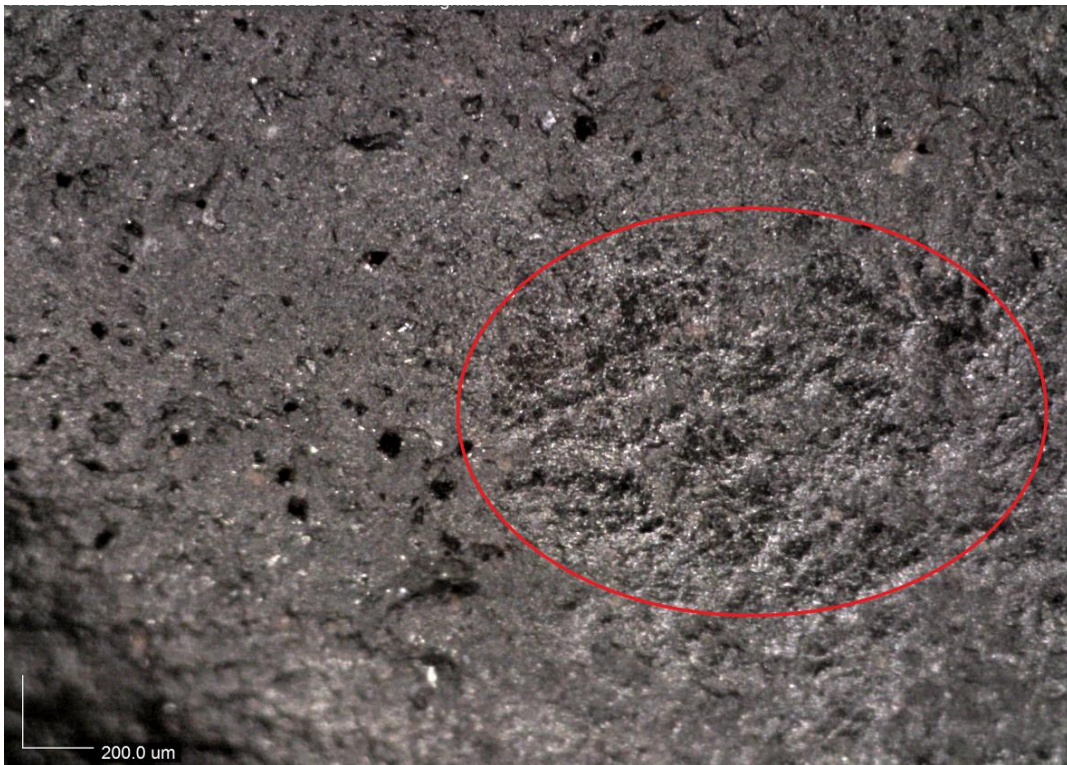
Figure 9.5. Acid hole created by the corrosion of the stone surface, DM OM 135x (Tool ID #VII 1880).
