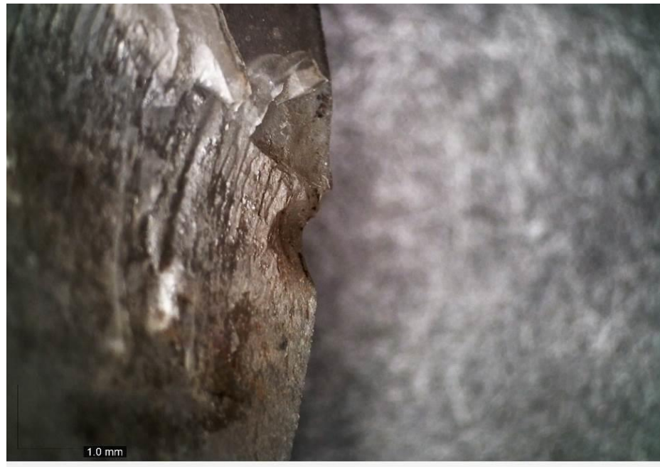
Figure 7.7. Edge-damage due to the presence of a hafting system. Scalar and triangular scars. A: dorsal right proximal side of the tool; B: ventral right proximal side of the tool. DM OM 40x (experiment code: TR-87).
