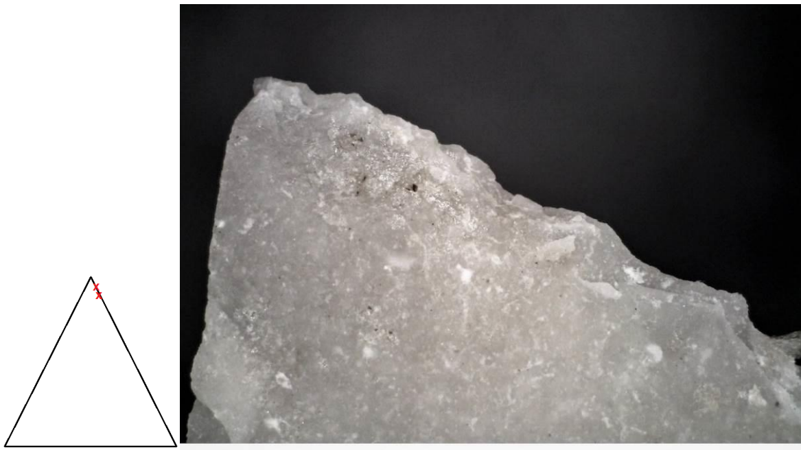
Figure 6.17. Intense edge-damage, i.e. tip-crushing. The tip is completely crushed after impact creating multiple cone scars, DM OM 50x (experiment code: TR-86).
