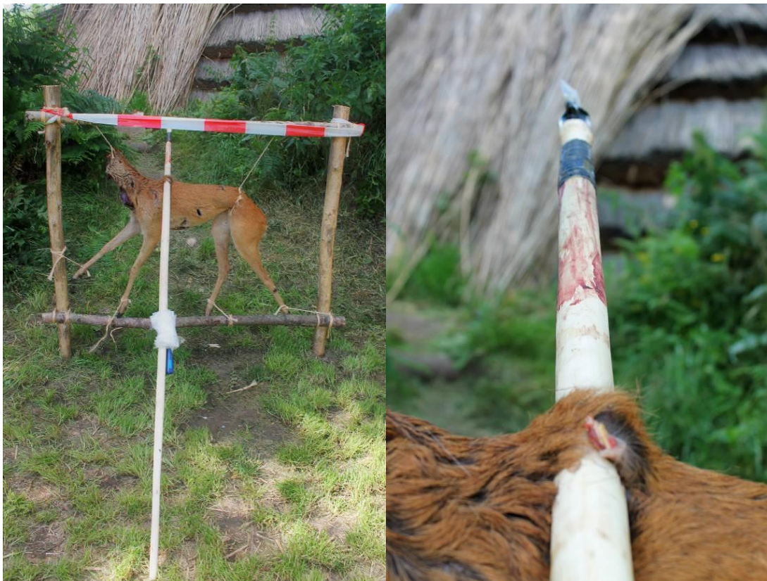
Figure 5.24. An example of a deeper penetration caused by a hand-delivered throwing stone-tipped spear (experiment code: TH-77).
