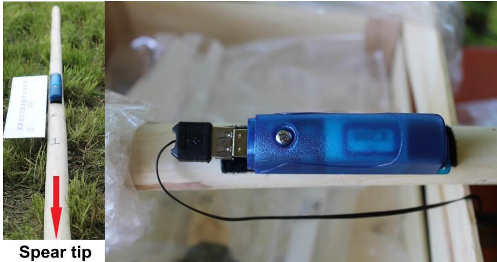
Figure 5.33. Position of the X200-4 accelerometer on the experimental spear shaft. (Image La Porta).
