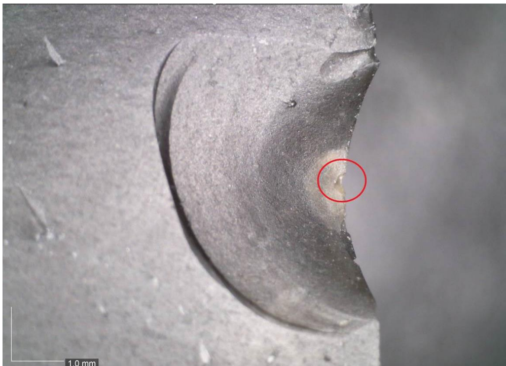
Figure 2.15. Cone scar with an indication of the point of impact (red circle), DM OM 40x.
