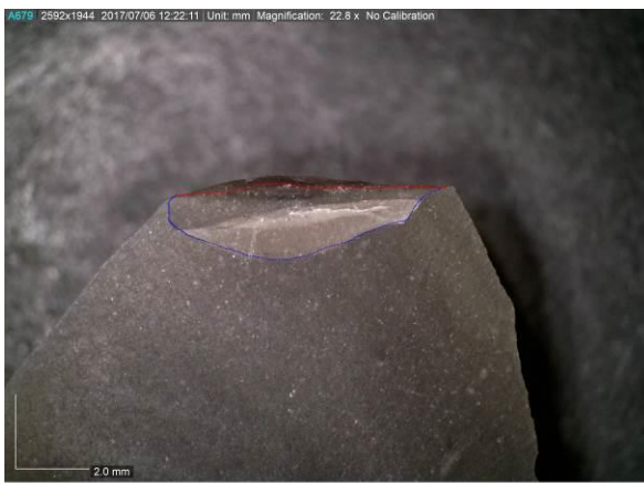
Figure 64. Location A (Form 27, Fig.1). Locus D1v: snap-terminating bending fracture (in red) plus unifacial spin-off fracture (in blue). OM/DM 50x.
