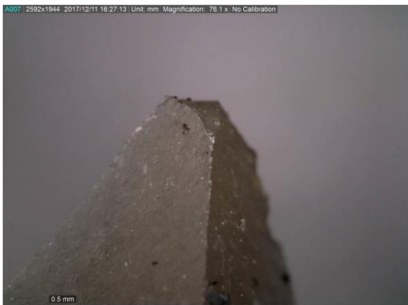
Figure 38. Location A (Form 16, Fig.1) Locus D1d: feather-terminating bending fracture DM/OM 76x.
