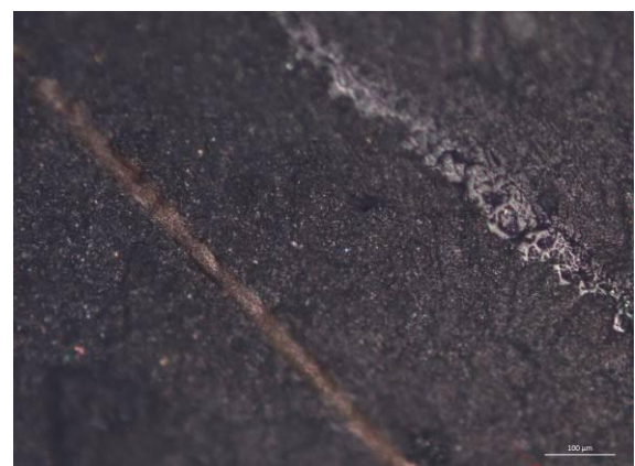
Figure 49. Location C (Form 20, Fig.1). Locus Pv1: tar deposit and tar additive layer, colour picture OLMil/OM 100x.
