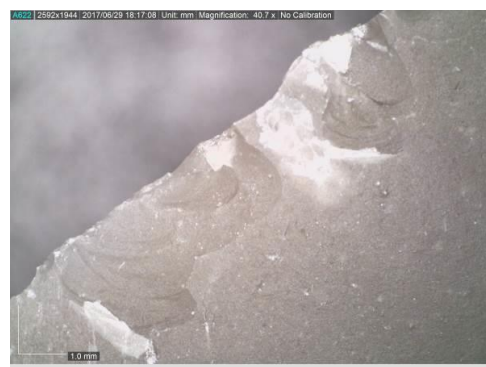
Figure 111. Location C (Form 46, Fig.1). Locus D2v: edge-damage, DM/OM 40x
