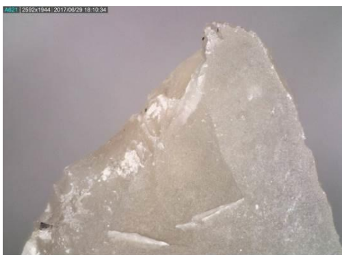
Figure 109. Location A (Form 46, Fig.1). Locus D1v: multiple fracture pattern, DM/OM 80x
