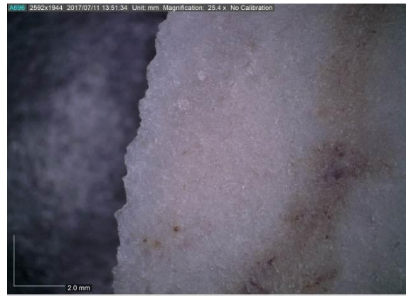
Figure 10. Location B (Form 3, Fig. 1). Locus D2v: denticulated edge-damage, DM/OM 25x.
