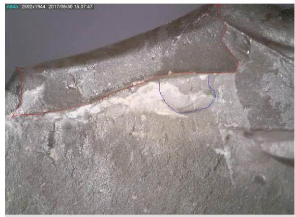
Figure 124. Location A. (Form 52, Fig. 1). Locus D2d: hinge bending fracture plus spin-off, DM/OM70x.
