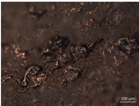
Figure 114. Location B (Form 48, Fig. 1). Locus P2v: tar residue, OM/OLM 100x
