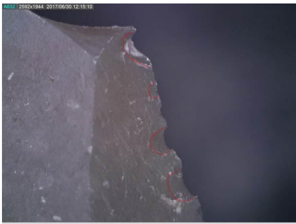
Figure 97. Location A (Form 38, Fig. 1). Locus D1d: edge-damage. Large scalar cone scars, DM/OM 50x.
