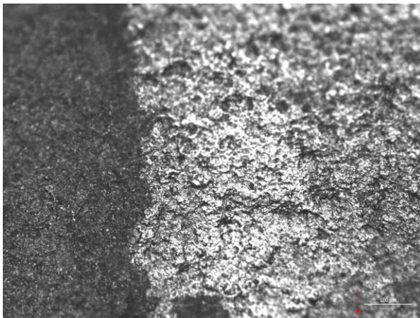
Figure 123. Location B. (Form 52, Fig. 1). Locus P1v: tar polish, OM/OLM 100x.
