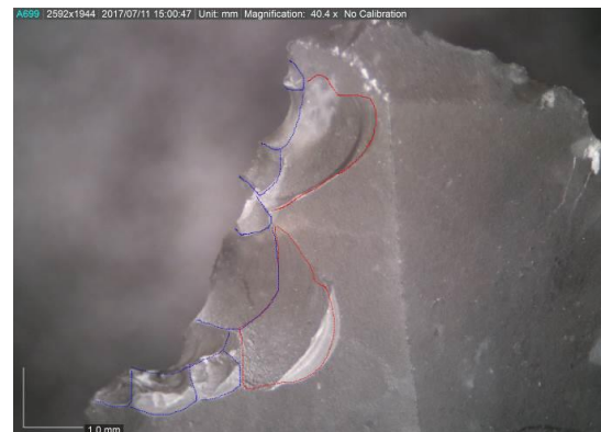
Figure 29. Location A (Form 11, Fig. 1). Locus D3d: pattern of multiple fractures, DM/OM 40x.
