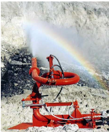
Figure 3.8 (left) A modern remote-control china clay monitor. Photo © The China Clay History Society
