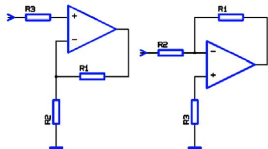
**Figure 3 – Eliminating the effect of bias current**
