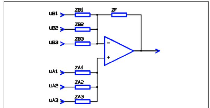
**Figure 4 – The Impedance Balancing Rule**
