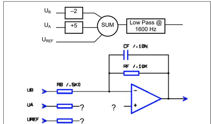
**Figure 1 – A "difficult" design of amplifier**
