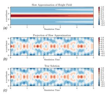
Figure 1: The time evolution of a 1D Gaussian dam-break problem using the psuedo-1D shallow water equations used in [5]. The figure is for  $\epsilon$ =0.005; (a) shows the evolution of the frequencyfiltered twist equation (3); (b) is the result of rotating (a) back using the matrix exponential mapping (2); and (c) the time-evolution of the dam-break problem computed with a 4th order runge-kutta timestepping method. Courtesy Adam Peddle.
