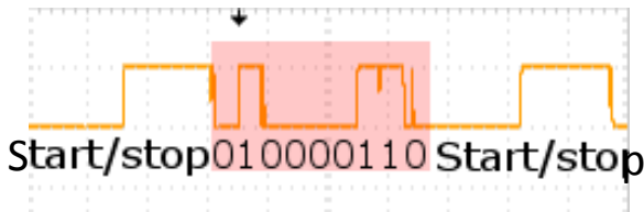
Fig. 10. Data transfer test "C" ASCII character (01000011) with 0 parity bit.
