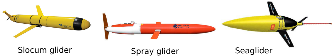
Figure 4.1.1: A Slocum glider, a Spray glider and a Seaglider
