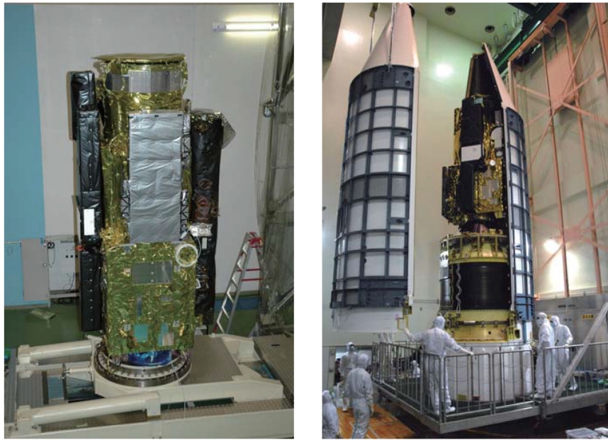
Fig. 1. Hinode spacecraft. On the left-hand-side panel, we can see EIS to the left and XRT to the right of the satellite body. At its center is SOT, with the focal-plane package (FPP) on our side. (Color online)
