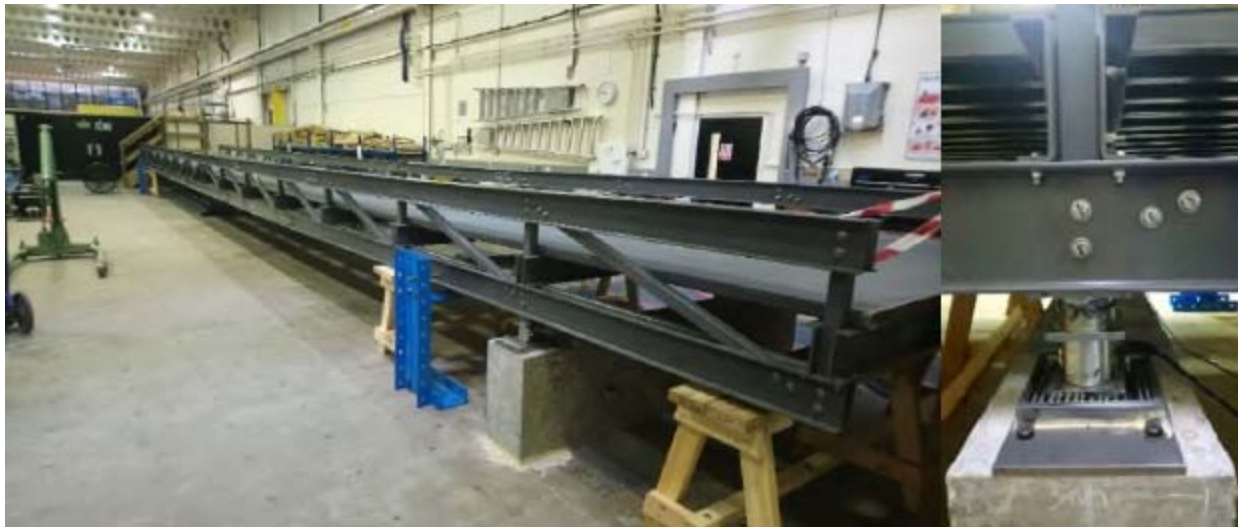
Fig 1 Photograph of the FRP Bridge. Left. Full view of the structure. Right. Support conditions
