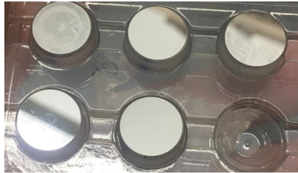
Figure 6.9. Photograph showing the non-uniform coverage and poor adhesion of the WS_2 films on the silver mirrors.
