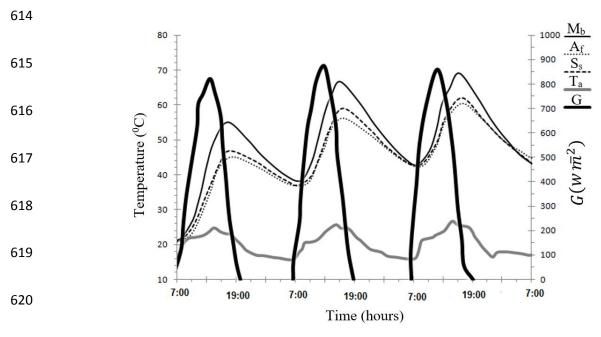
Fig. 5 - Temperature changes for three consecutive days ( $M_b$ : Mirror booster ,  $A_f$ : Aluminum foil,  $S_s$ : Steal sheet,  $T_a$ : ambient temperature , G: incoming solar radiation intensity)
