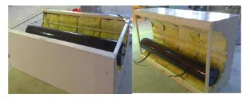
Fig. 3: Construction and assembling the ICS SWH system
