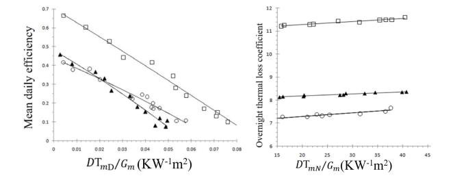
Fig. 6 – Overnight thermal loss coefficients and mean daily efficiency  $(M_b: \Box, A_f: \circ, S_s: \blacktriangle)$
