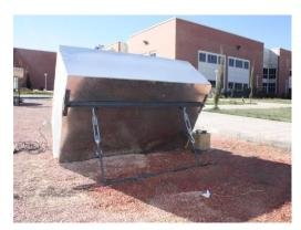
Fig. 4: The constructed ICS SWH at the testing site in Kerman
