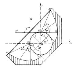
Fig. 2: Cross-section view of a symmetric CPC [22]
