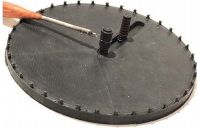
Fig. 1. Experimental setup of superdirective dimer. Copper helices are wired around PLA base ( \epsilon = 2.6 ). Resonant frequency f_0 = 1.53 .
