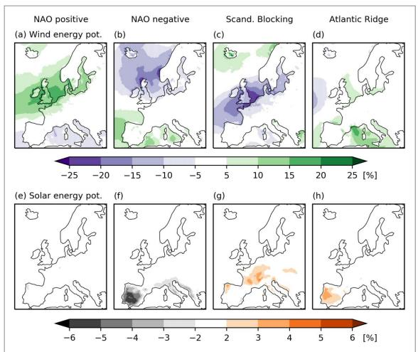
**Figure 3.** As figure 2 but here for mean power production impacts of the four weather regimes. Colours show anomalies of (a)—(d) wind power potential (%), (e)—(h) solar power potential (%). Each weather regime in a column, labelled at the top, left to right: NAO positive, NAO negative, Scandinavian Blocking, Atlantic Ridge. Figure based on ERA5 data (DJF, 1979–2018).
