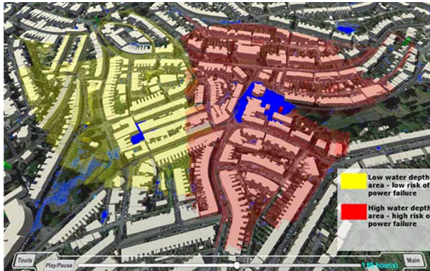
Figure 18 | Substation failures and dependent power outage areas. In yellow are the areas with small risk of the power failure and small water depth. In red are the areas with high risk of the power failure and high water depth. Please refer to the online version of this paper to see this figure in colour: http://dx.doi.org/10.2166/hydro.2019.032 .
