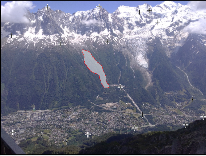
Figure 5: Terrestrial oblique image MB-O18 of the Chamonix valley, showing the general terrain configuration, the control points for camera orientation and calibration, as well as the polygonal feature used for the inverse perspective validation.
