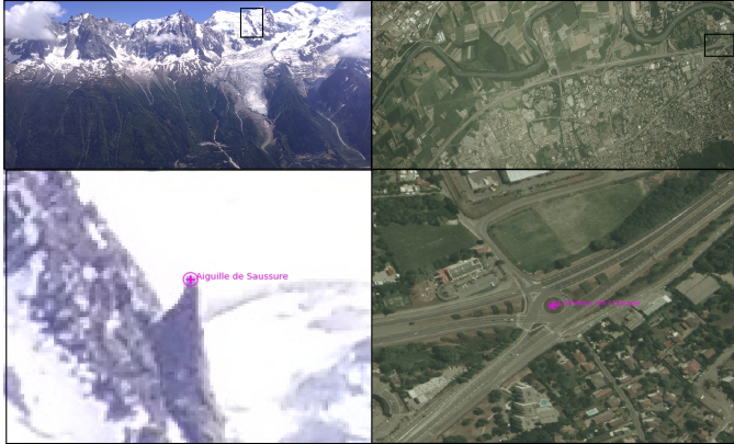
Figure 7: Example of definition of 2D control points for the MB (left) and G (right) case studies. The two lower panels are zooms of the upper row. Circles represent the 90% confidence radius, accounting for the user’s judgment on point uncertainty.
