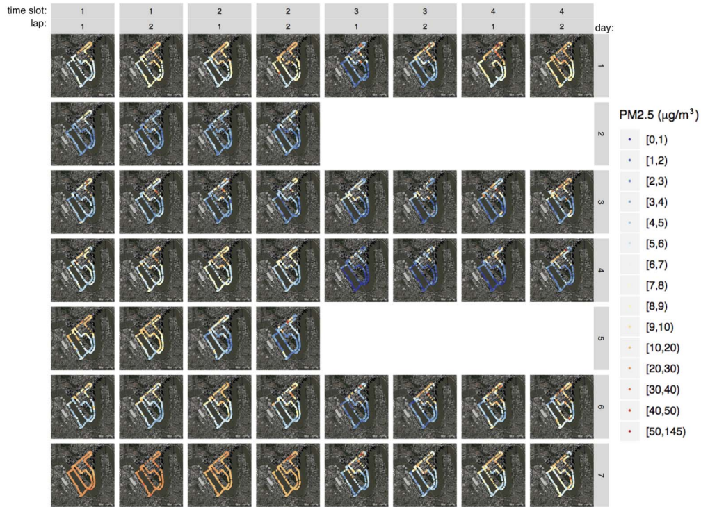
Figure 3: The 48 PM 2.5 laps of data collected using the KOALA mobile air quality monitor. These 48 laps were collected over 24 time slots, (1–4) on weekdays and (1–2) on weekends [columns], and 7 days in May 2018 (Thursday 10/05/2018, Sunday 13/05/2018, Tuesday 15/05/2018, Thursday 17/05/2018, Sunday 20/05/2018, Tuesday 22/05/2018, Thursday 24/05/2018) [rows].
