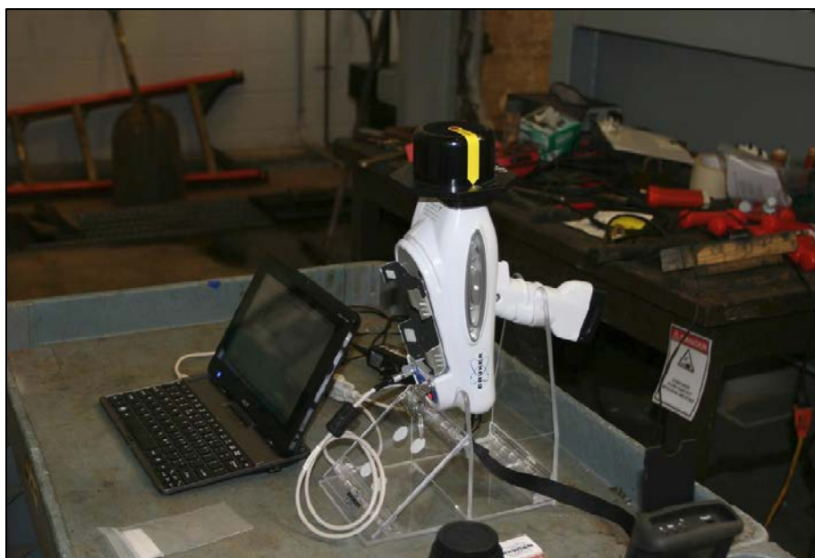
Figure 9.7 Bruker Tracer III-SD handheld (pXRF) x-ray fluorescence spectrometer system (Rusch 2013).
