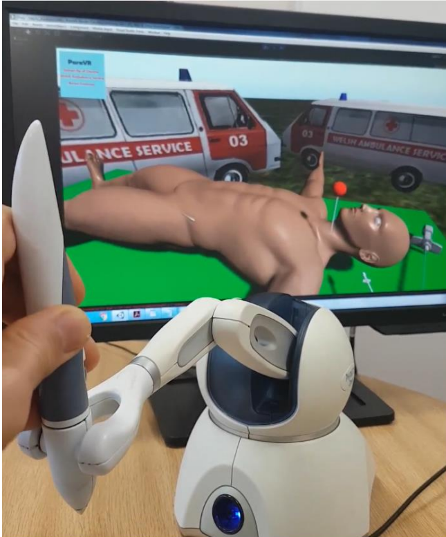
Figure 3. Geomagic Omni 6-DOF Haptic Device with the ParaVR simulator of Needle Cricothyrotomy.
