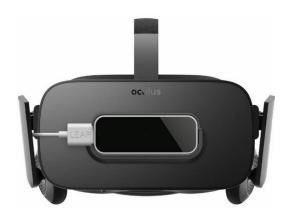
Figure 2. Leap Motion Hand Tracking sensor on the Oculus Rift HMD.
