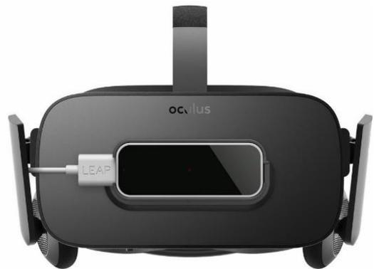
Figure 2. Leap Motion Hand Tracking sensor on the Oculus Rift HMD.
