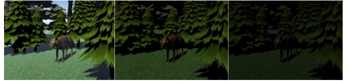
Fig. 7. The developed VR 3D Scene of a spruce forest containing predators at various light levels. This provides one of the custom fabricated datasets for image classification to evaluate the evolving eyes.
