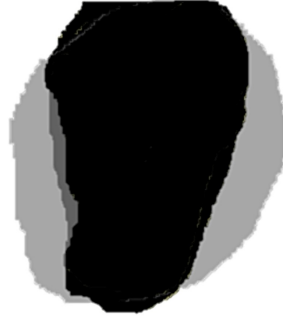
Figure 8: Changes in particle shape with temperature for PEK HP3. The darkest image corresponds to the particle at room temperature, followed by the particle at t^* = 0 and the lightest colour corresponds to the particle at t_{\text{end}}^*
