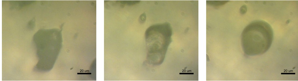
Figure 6: Hot Stage Microscopy images for individual particles of PEK HP3. An individual unit of coalescence evolves in time to minimise the surface area. The surface roughness elements flatten and particle reaches an overall spherical shape. The figures correspond to room temperature, t^* = 0 and t_{\text{end}}^* from left to right.
