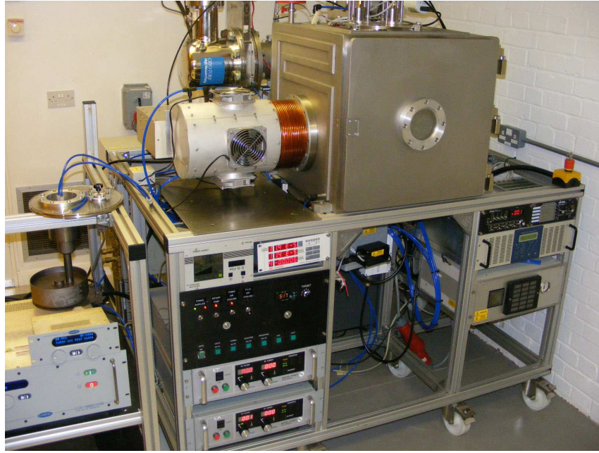
Figure 2.15: Photograph showing the HiTUS system used for the deposition of the coatings in this work.
