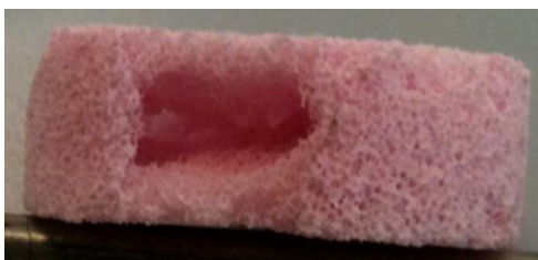
Fig. 6. 5. Hollow ceramic foam produced by the supplier.
