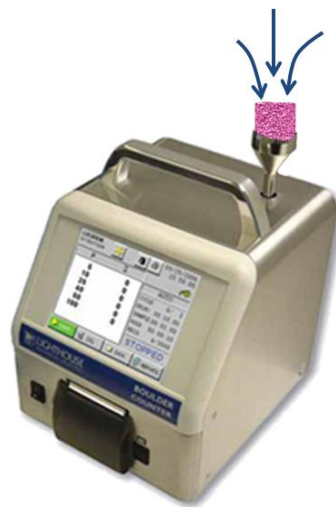
Fig. 6. 10. Lighthouse portable airborne laser particle counter (SOLAIR 3100) with filter placed on its inlet.
