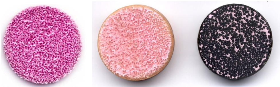
Fig. 5. 2. Photograph of a plain ceramic matrix (left) before and after polymer infiltration (middle), and the ceramic-CNT-epoxy resin composite (right).
