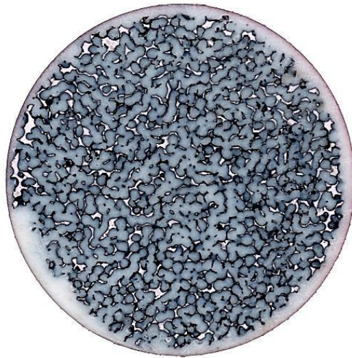
Fig. 5. 9. Photograph of the polished surface of a polyamide-ceramic-CNT composite. Black curves, grey parts and white bright parts are contributed to the CNT, PA12 and ceramic, respectively. The interconnectivity feature of the pores is also visible in this photo.
