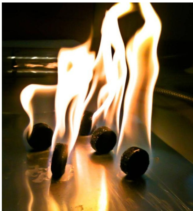
Fig. 6. 6. Several filters burning after filtration of yeasts by adding acetone, representing a method for the filter regeneration.
