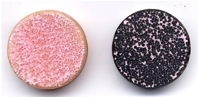
Fig. 3. 11. Photograph of samples after polishing without (left) and with (right) CNTs.
