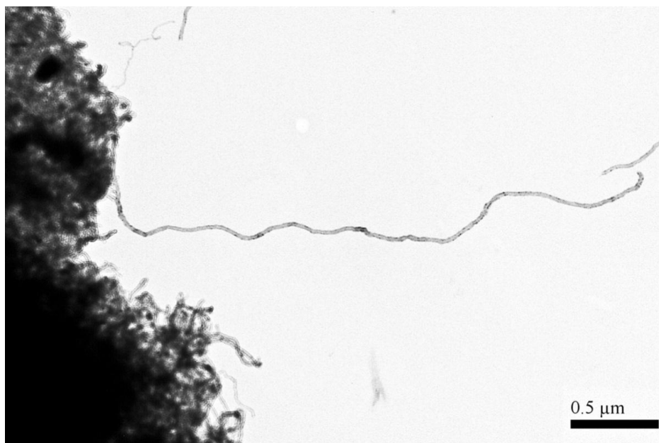
Fig. 4. 35. TEM image shows the length of a CNT.
