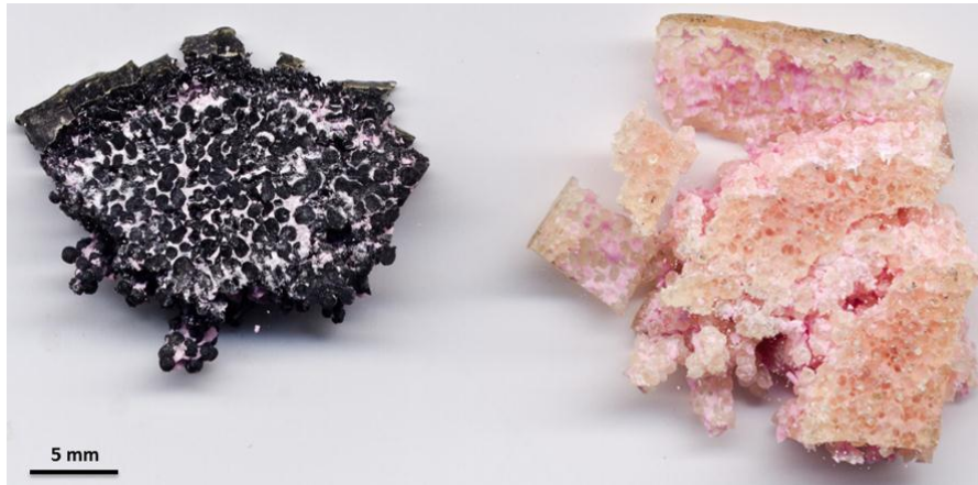
Fig. 7.2. Optical image of the compressed samples where the left one is the epoxy resin-ceramic-CNT composite and the right one is the epoxy resin-ceramic one.
