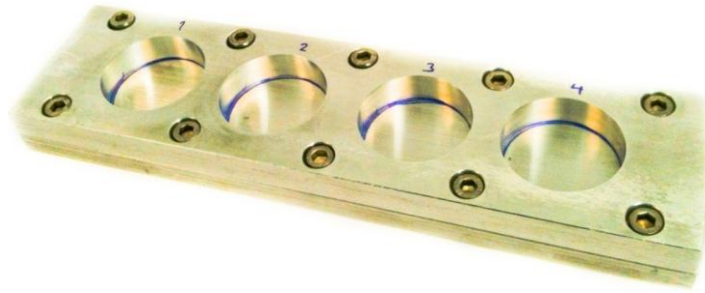
Fig. 3.16. The specially designed mould for increasing the diameter of the composite samples (located in the middle of the holes) by adding an extra epoxy resin ring around the central composites.
