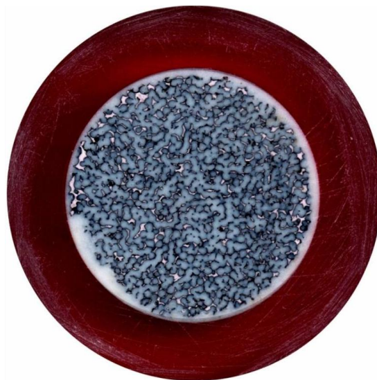
Fig. 3. 17. Optical image of PA12-ceramic-CNT composite after increasing its diameter by the addition of epoxy resin for impact test.
