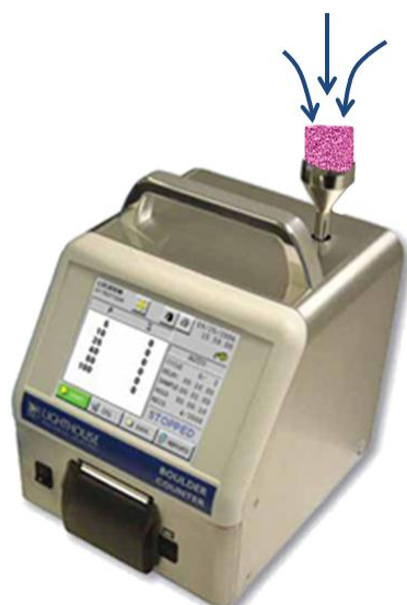
Fig. 3.7. Lighthouse portable airborne laser particle counter (SOLAIR 3100) with filter placed on its inlet.
