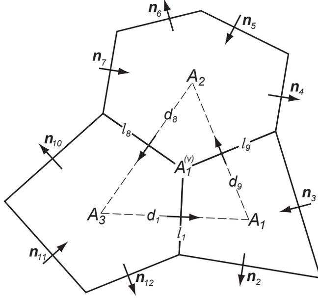
Fig. 2. Schematic showing the geometrical information needed to define a C-grid scheme on an arbitrary polygonal grid: primal edges are shown by continuous lines and dual edges by dashed lines;  $l_e$  is the length of primal edge  $e$ ;  $d_e$  is the length of dual edge  $e$ ;  $A_i$  is the area of primal cell  $i$ ;  $A_v^{(v)}$  is the area of dual cell  $v$ ;  $\mathbf{n}_e$  is the unit normal at edge  $e$  indicating the direction corresponding to positive  $u_e$ .
