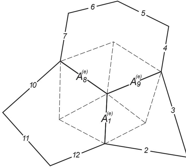
Fig. 5. Schematic showing the areas  $A_1^{(e)}$ ,  $A_9^{(e)}$ , and  $A_8^{(e)}$  associated with edges 1, 9, and 8. The area associated with edge 1 comprises the two triangles either side of edge 1.
