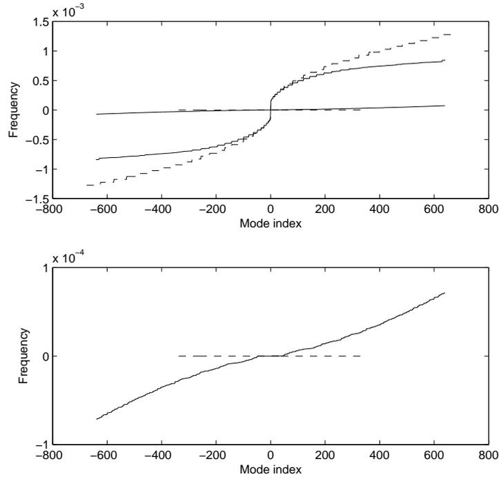
Fig. 9. Normal mode frequencies on the  $f$ -sphere. The upper panel is like the upper panel in Fig. 8 but for a scheme that reduces to the scheme used by [16] on a plane regular hexagonal grid. The lower panel shows the same data but with a much expanded frequency scale to make clear the non-zero frequencies of the geostrophic modes.
