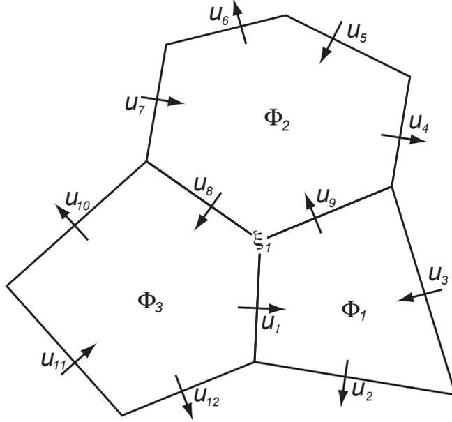
Fig. 3. Schematic showing the locations of the prognostic variables  $\Phi_i$  and  $u_e$ , as well as the natural location for diagnosing the relative vorticity  $\xi$  at vertex 1.
