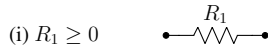
Fig. 1. Network N_1 . We define \mathcal{N}_1 as the set of all networks of the form of N_1 that satisfy condition (i).
