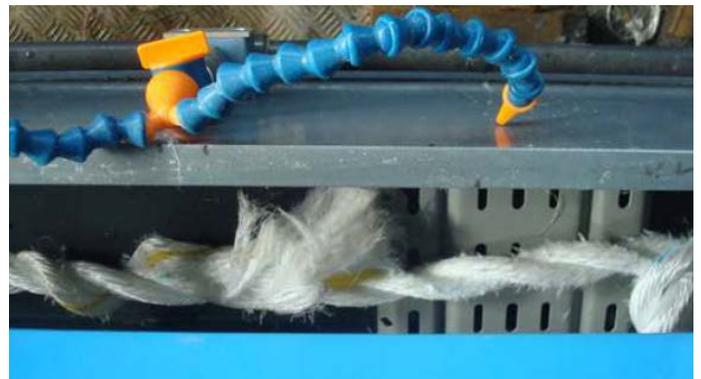
(c) 3 broken strands at end of eye (Test 02) at IFREMER
