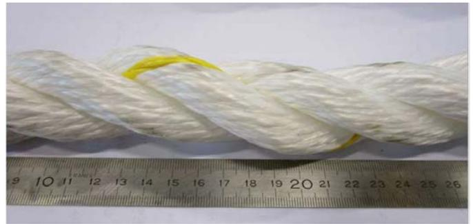
**Figure 1. Test specimen for RRT: EUROFLEX® 3 Strand rope manufactured by Lankhorst Ropes.**
