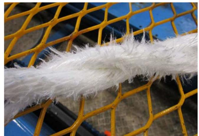
(d) Furring of rope near failure zone
