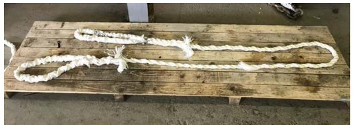
(b) 1 broken strand near end of splice (Test 02) at DMaC
