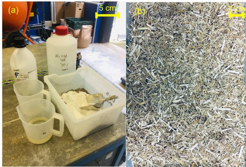
Fig. 1. Initial and raw materials: (a) Powder precursors and liquid alkali-activators, (b) Miscanthus particles
