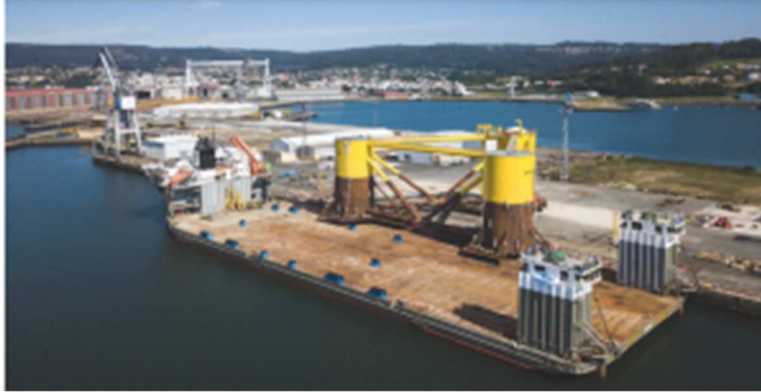
Figure 1 Loadout of semi-submersible onto a heavy transport vessel (courtesy Principle Power)
