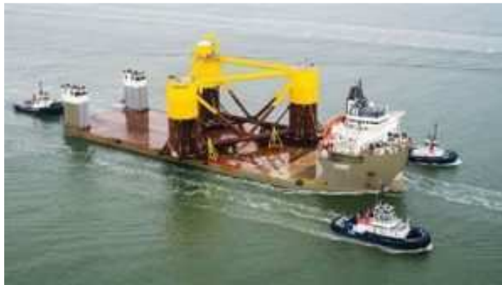
Figure 2 Ocean delivery voyage of a semi-submersible substructure (courtesy Principle Power)
