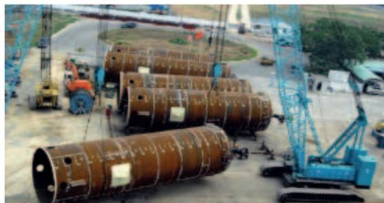
Figure 8 Suction pile anchors [14]
