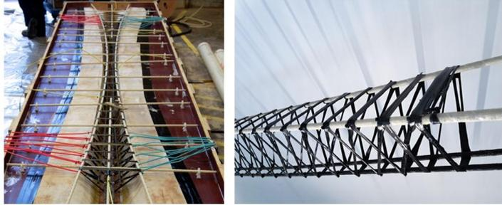
(b) Reinforcing shape optimised concrete beams with wound FRP cages (Spadea et al. (2016))
