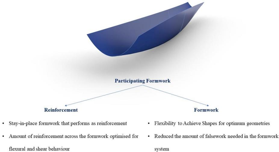
Fig. 3 Conceptualisation of participating formwork for shape-optimised concrete beams
