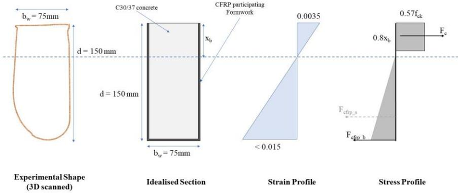
Fig. 5 Idealised stress and strain profiles for flexural analysis
