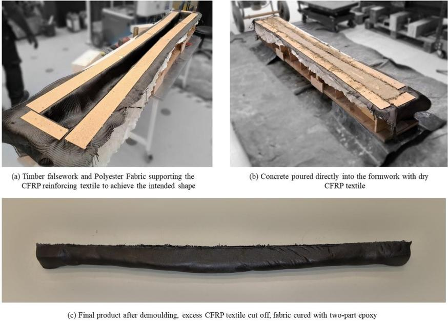
Fig. 4 Construction process of the shape-optimised beam with CFRP participating formwork
