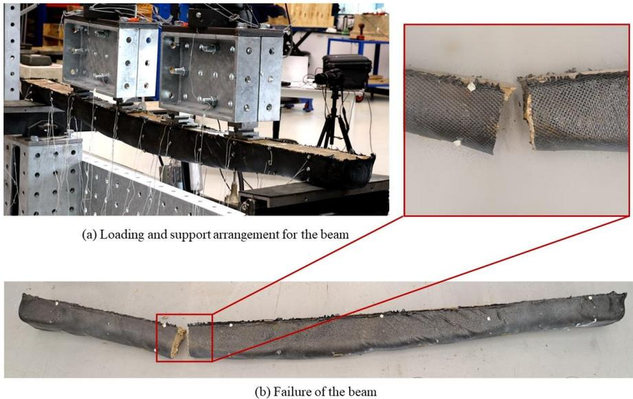
Fig. 6 Testing and failure of the prototype beam
