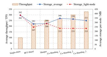
Fig. 3. Comparison of throughput and storage overhead.
