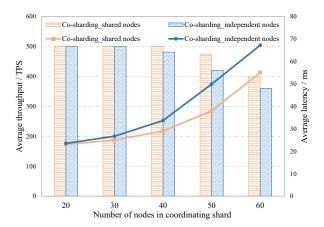
Fig. 6. Comparison of performance with the number of nodes in coordinating shard.
