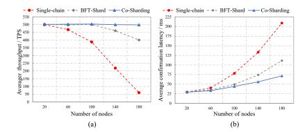
Fig. 4. Comparison of cross-region data retrieval performance with workload. \*(a) Throughput (b) Latency
